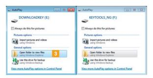
3 The operating system opens two dialogue boxes. Here you can choose the programme to be used for displaying the contents of the drive. If an SDHC<sup>™</sup> card is inserted, three dialogue boxes will be displayed.
