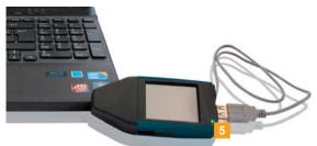
5 Check that the data transfer to and from the DLKPro has finished: The LED light remains green.
